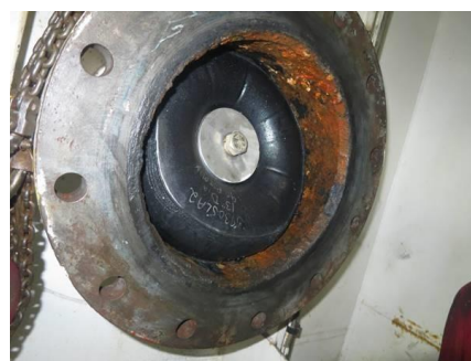
Valve Isolation with ROV Deployed ODIN Plug
