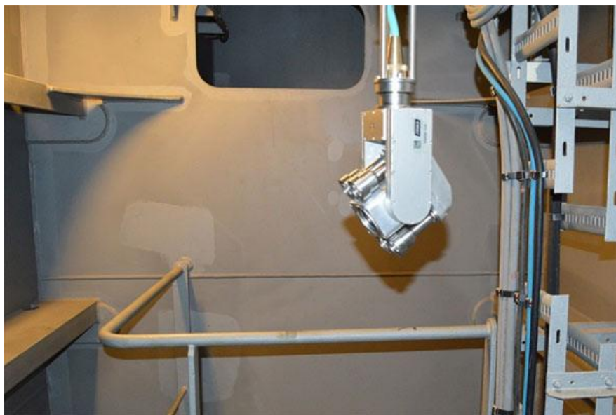
Figure 3. The NoMan camera can pan, tilt and zoom.
